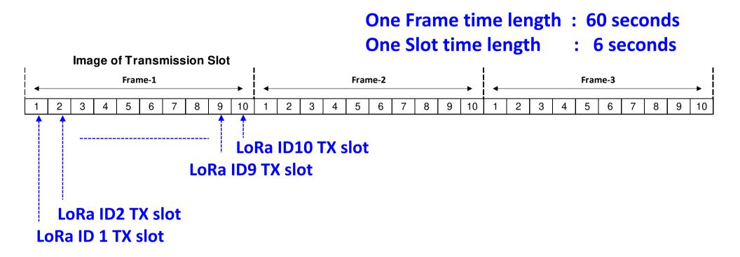
Each radio station assigned LoRa ID 1 to 10 is allowed to transmit only to its own ID number slot. This avoids transmission collisions and realizes reliable radio communication.
